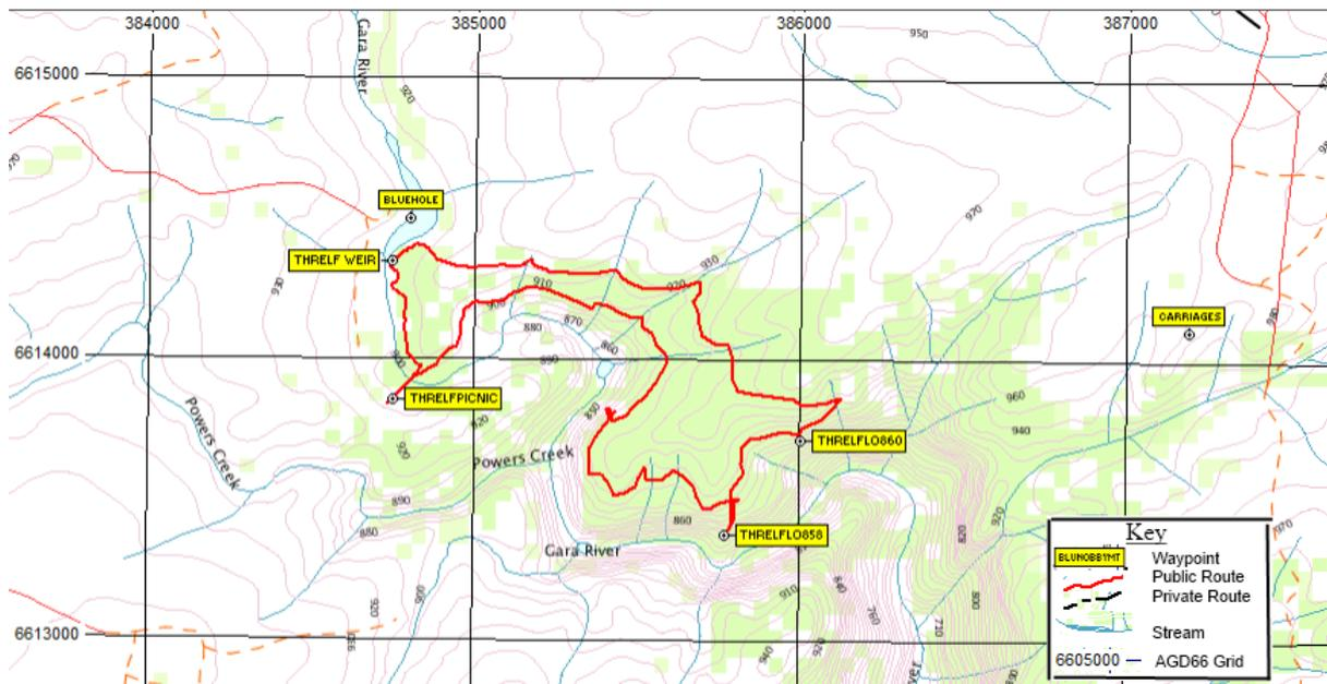
The maps used on the site generally have a 1 km grid. To give a full grid reference to the nearest metre (using say Threlfall Picnic area), then
